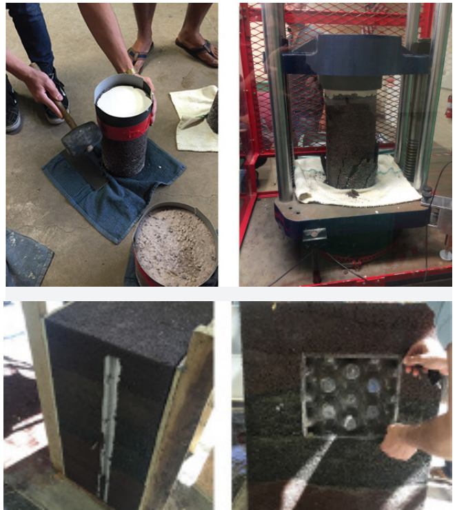
Figure 3. Cylinder tests and wall mockups. Photos by author..
